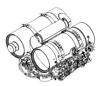
Illustration 21 g02446896 View of the exhaust system of a C13 Well Service Engine
