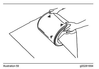
Do not use paint, a waterproof cover, or plastic as a protective covering for storage. An air flow restriction may result. To protect against dirt and damage, wrap the primary air cleaner elements in Volatile Corrosion Inhibited (VCI) paper.
