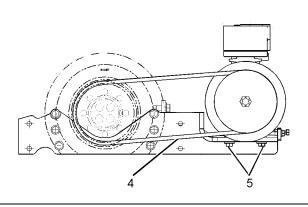
Illustration 45 (4) Drive belt for the air compressor (5) Mounting bolts g01389673
