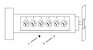
Illustration 17 Cylinder and valve location (A) Exhaust valve (B) Inlet valve g01387009
