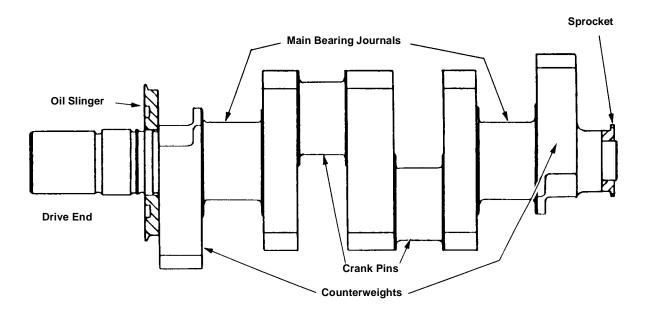
FIGURE 5-8: CRANKSHAFT - TYPICAL STUBSHAFT
