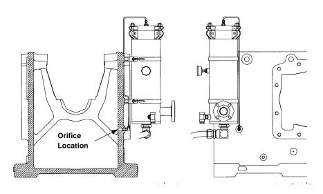
FIGURE 4-10: JGE/6 OIL FILTER FLOWING VENT TO PREVENT AIR ENTRAPMENT
