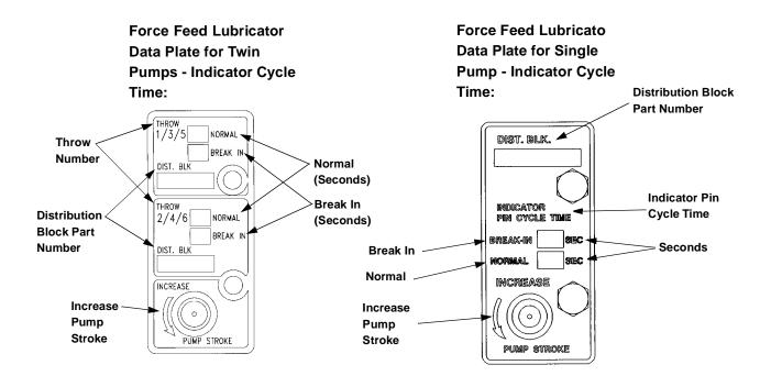
FIGURE 1-5: FORCE FEED LUBRICATOR DATA PLATES
