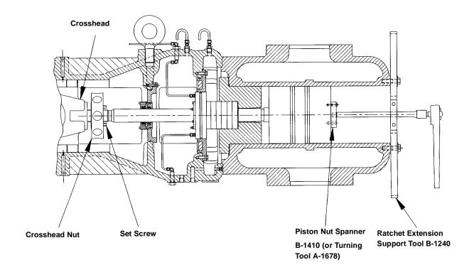
FIGURE 5-19: PISTON AND ROD INSTALLATION - TYPICAL
