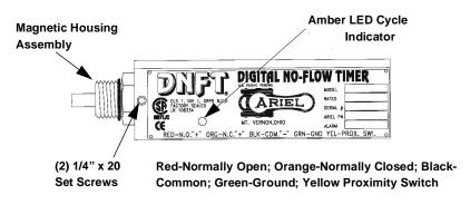
FIGURE 4-4: DIGITAL NO-FLOW TIMER SWITCH - (DNFT)
