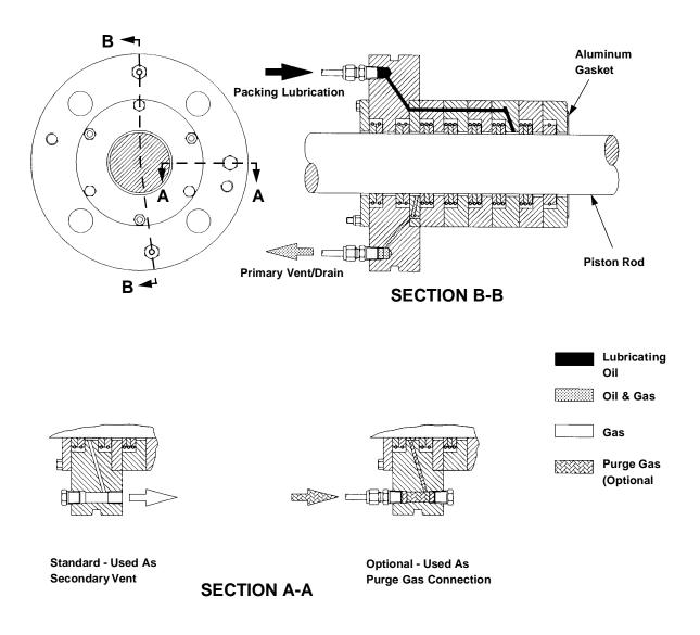
FIGURE 4-15: PACKING LUBRICATION AND VENTING - SINGLE COMPARTMENT DISTANCE PIECE
