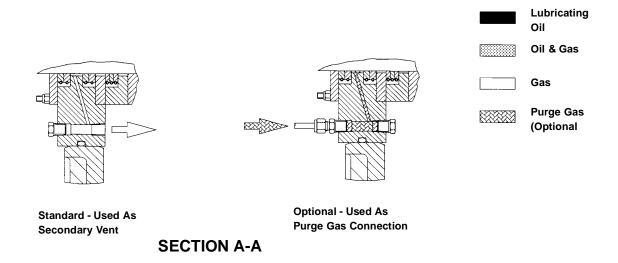
FIGURE 4-16: PACKING LUBRICATION AND VENTING - DOUBLE COMPARTMENT DISTANCE PIECE
