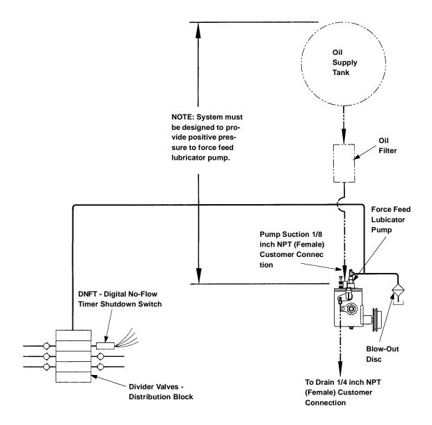
FIGURE 4-8: FORCE FEED LUBRICATION SYSTEM - INDEPENDENT OIL SUPPLY
