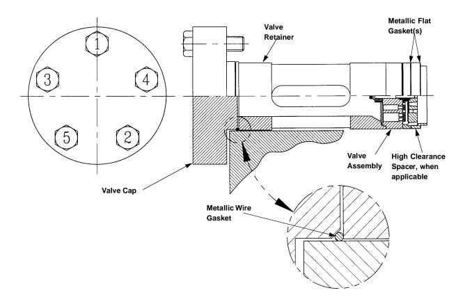
FIGURE 5-28: HIGH PRESSURE VALVE CAP ASSEMBLY
