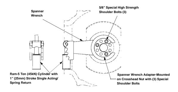
FIGURE 5-6: OPTIONAL HYDRAULIC CROSSHEAD-NUT TORQUING TOOL, G-7583
