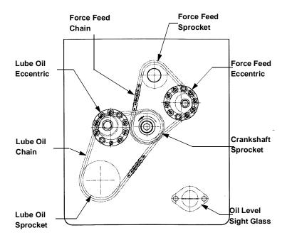
FIGURE 5-12: CHAIN DRIVE SYSTEM JGE/6 - TYPICAL (STANDARD ROTATION)
