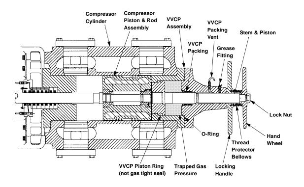
FIGURE 5-29: CYLINDER WITH VVCP - TYPICAL
