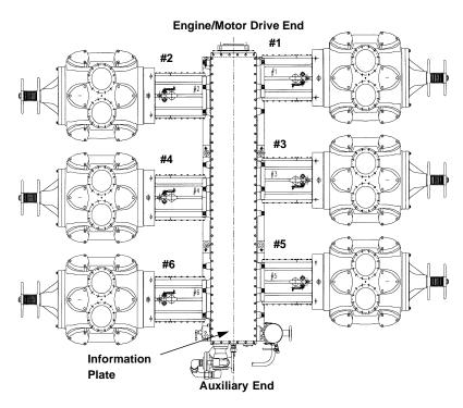
FIGURE 1-1: TYPICAL COMPRESSOR THROW NUMBERING AND INFORMATION PLATE LOCATION
