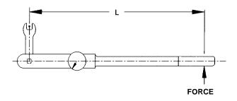
FIGURE 1-12: TORQUE WRENCH WITH ADAPTOR AT RIGHT ANGLE
