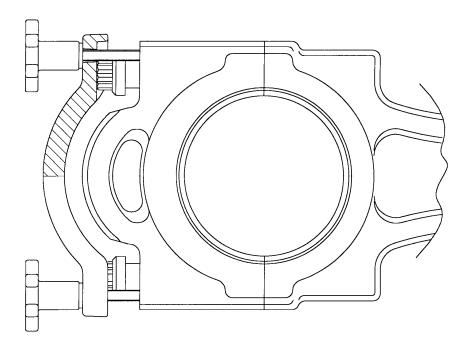
FIGURE 7-2: CONNECTING ROD CAP REMOVAL TOOL - TYPICAL (C-2106)
