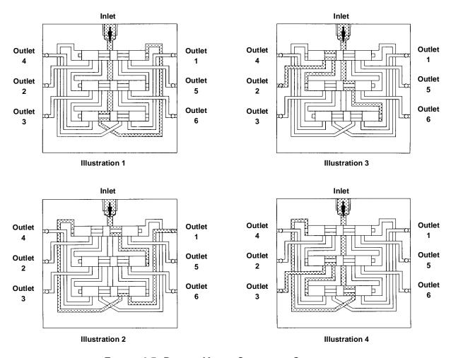
FIGURE 4-5: DIVIDER VALVE OPERATION SCHEMATIC
