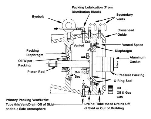
FIGURE 4-14: SHORT-TWO COMPARTMENT DISTANCE PIECE - PACKING, TUBING & VENTING
