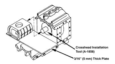
FIGURE 5-3: CROSSHEAD INSTALLATION
