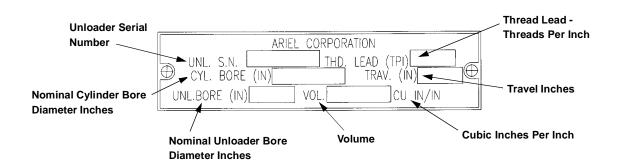
FIGURE 1-7: CYLINDER AND UNLOADER IDENTIFICATION PLATES
