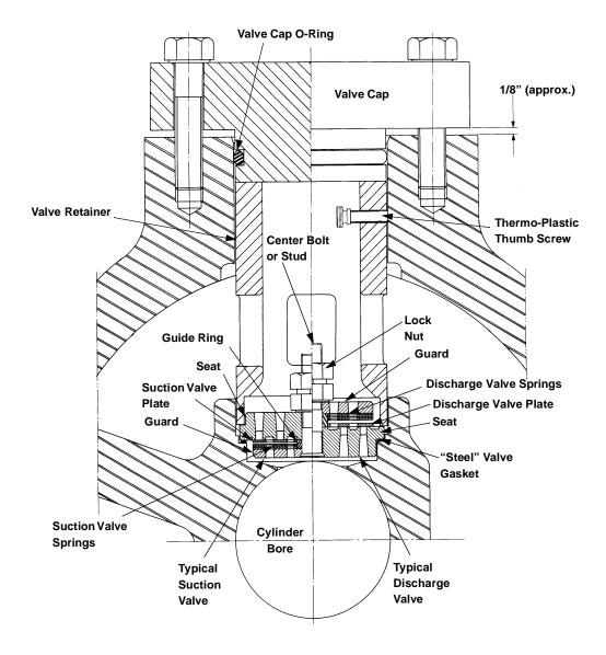
FIGURE 5-27: TYPICAL VALVE ASSEMBLIES
