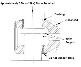
FIGURE 5-4: CROSSHEAD BUSHING REPLACEMENT
