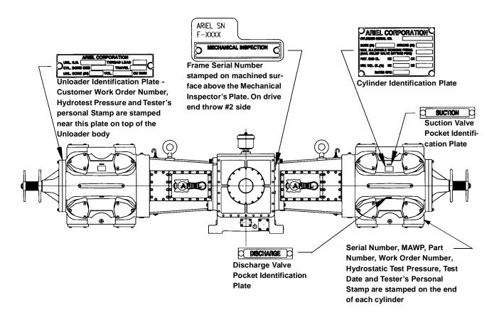
FIGURE 1-6: IDENTIFICATION PLATES - TYPICAL
