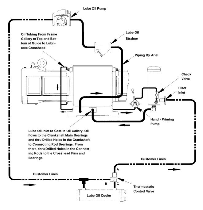
FIGURE 4-9: LUBE OIL SYSTEM SCHEMATIC
