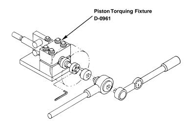
FIGURE 5-17: PISTON AND ROD CLAMPING REQUIREMENTS
