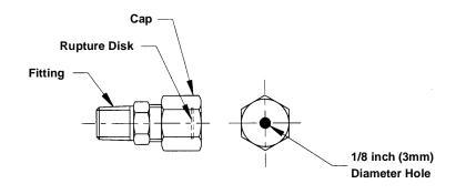
FIGURE 4-2: LUBRIQUIP BLOW-OUT FITTING ASSEMBLY
