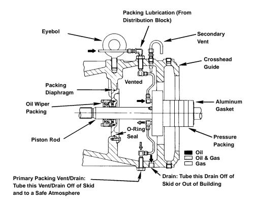
FIGURE 4-13: SINGLE COMPARTMENT DISTANCE PIECE - PACKING, TUBING & VENTING
