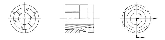
FIGURE 5-16: FENNER DRIVE COUPLING
