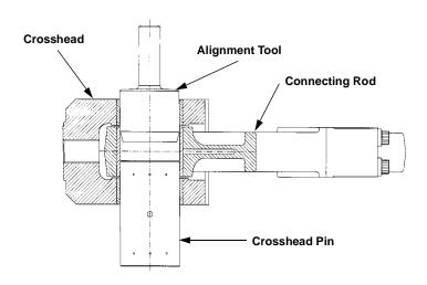
FIGURE 5-5: CROSSHEAD PIN ALIGNMENT TOOL (B-1989) - TYPICAL
