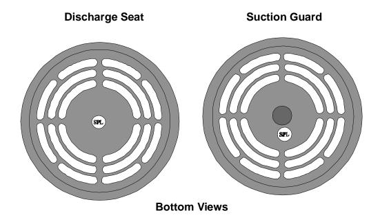
FIGURE 1-9: SPIRALOCK THREADED VALVE ASSEMBLY - MARKED "SPL"
