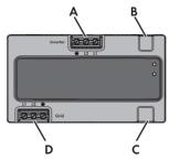
Figure 15: Connection areas on the Sunny Multigate
