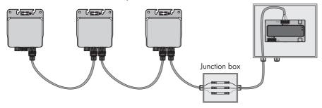
Figure 19: AC cabling of the entire PV system with junction box
