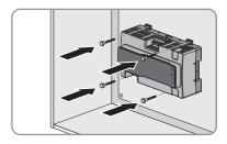
6. Make sure that the Sunny Multigate is securely in place.
