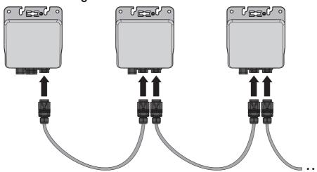
Figure 16: AC cabling among the inverters (left = last inverter; right = first inverter)
