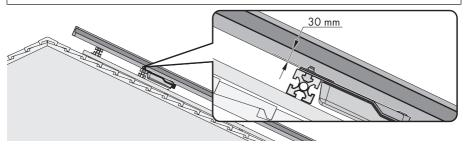
Figure 10: Minimum clearance of the inverter to the bottom side of the PV module
