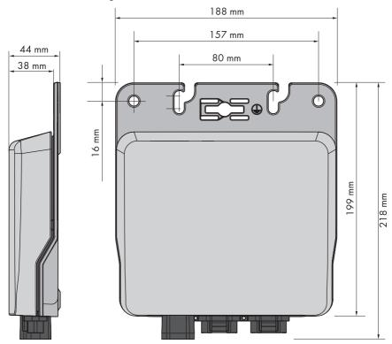
Figure 8: Position of the anchoring points
