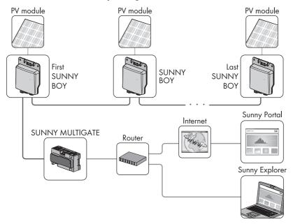
Figure 7: Example of a PV system with micro inverters and Sunny Multigate with communication via Speedwire/ Webconnect
