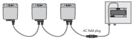
Figure 18: AC cabling of the entire PV system with AC field plug
