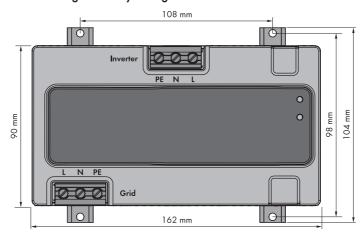
Figure 13: Dimensions of the Sunny Multigate and the drill holes for mounting with screws
