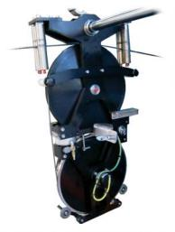
Innovative concept replacing remote load cell system at wellhead sheave pulley, the MP16 II can operate at variable rig up angles reducing K-Factor error. Wire oil lubricator tank is fitted to measure head. Can accept pressure transducer on tension load cell circuit for digital signal to Automation Products system. Can accept optical encoder on depth measuring wheel for digital signal to Automation Products system.
