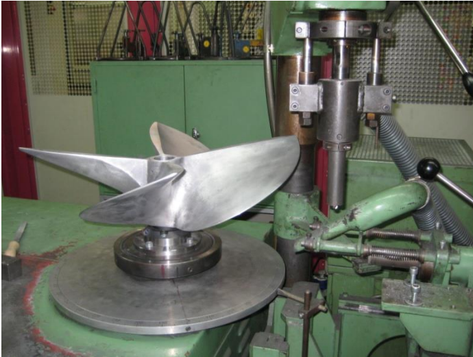
-Here a 24 inch Levi Diamond propeller in dynamic balancing machine
